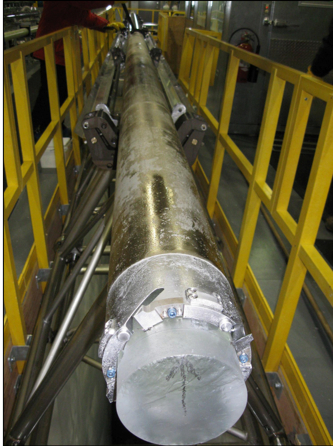
Figure 13. Recently drilled ice core sticking out of the drill sonde. An arrow identifies its original orientation in the ice sheet. [Photo by Peter Neff/U.S. IDP ]
