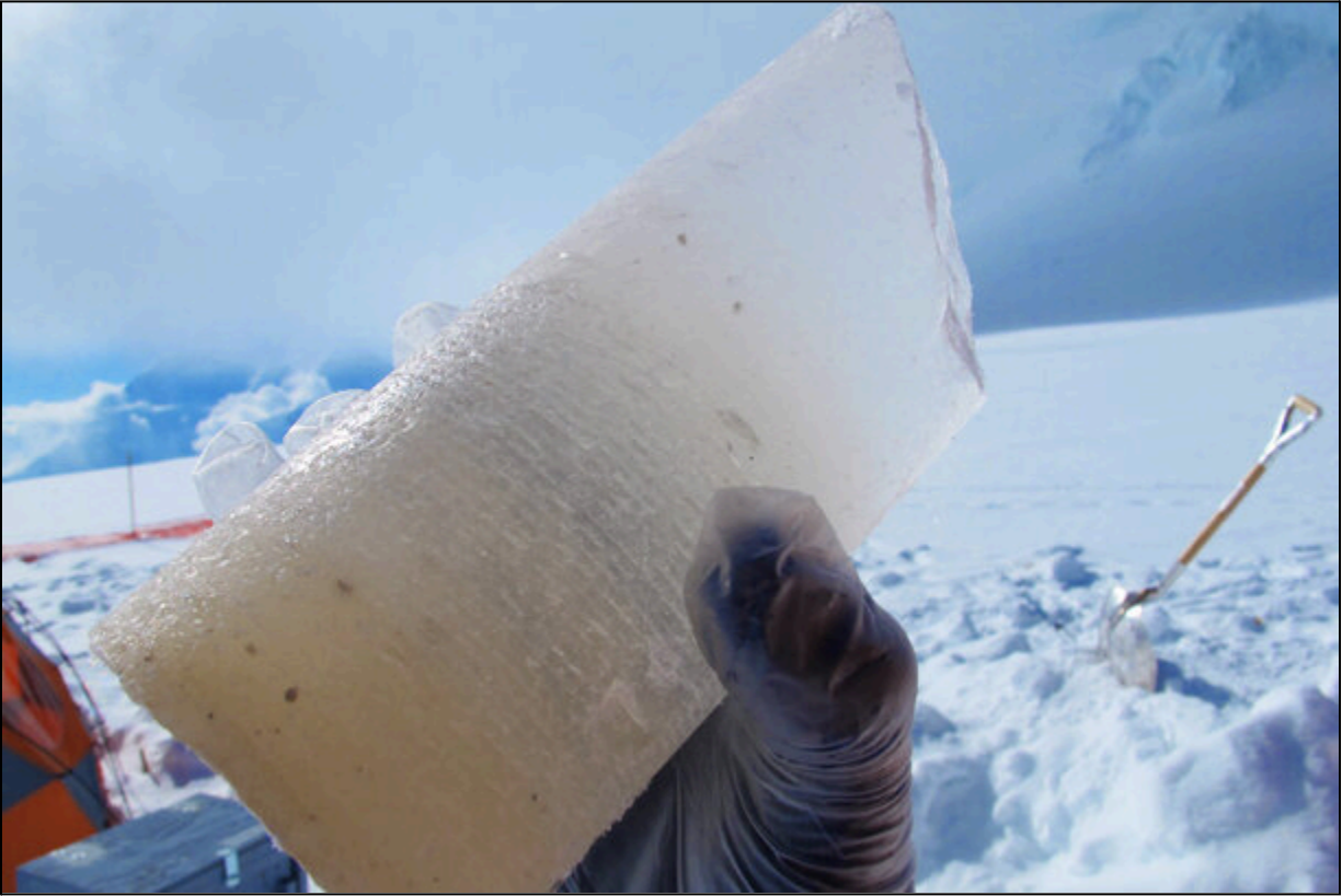
Figure i. The bottom of an ice core drilled in Alaska shows pebbles and dingy ice, indicating the presence of nearby bedrock. [Photo by Mike Waszkiewicz ]
