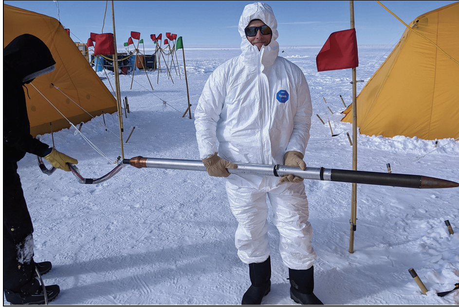
Figure 11. A scientist testing the ice diver on the Greenland ice sheet. The tip of the ice diver is metal and contains thermal wiring that melts quickly through the ice. [Photo from Dale Winebrenner/University of Washington ]
